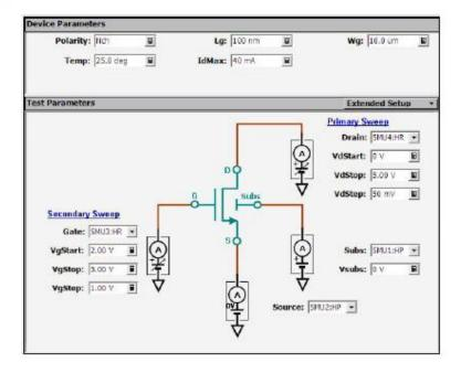
Recall Id-Vd application test setup data.
